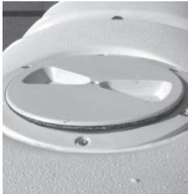
2. The transom drain bungs can be found on each hull next to the lower rudder pintle. (figure 2)
